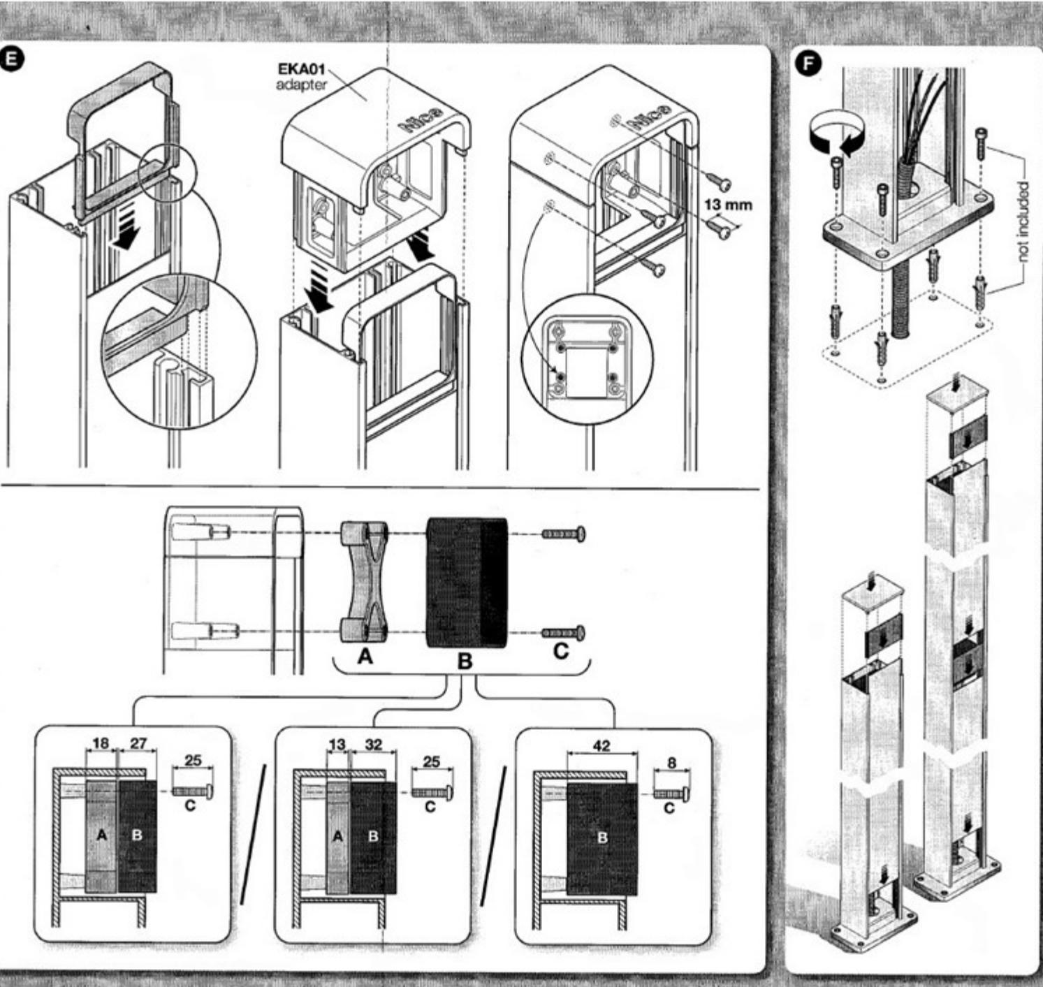
**Fig. A** - Fixing of the photocells of the "Era" series, by Nice.
